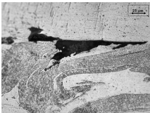
Fig. 8 Particular of the tunnel in the nugget, 15×
